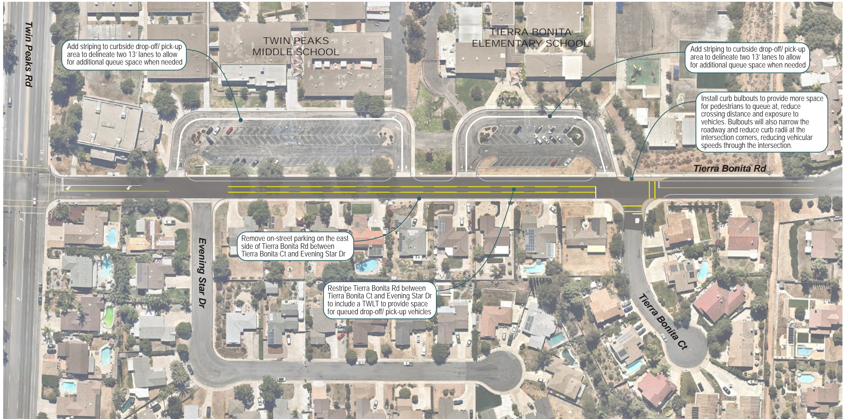
FIGURE 10- Preliminary Improvements along Tierra Bonita Road
